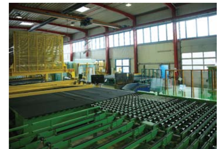
Fig. 02: Transported 'around the corner', the glass stream from laminated cutting is directly integrated in the sorting system. In the background: laminated glass Remaster.
