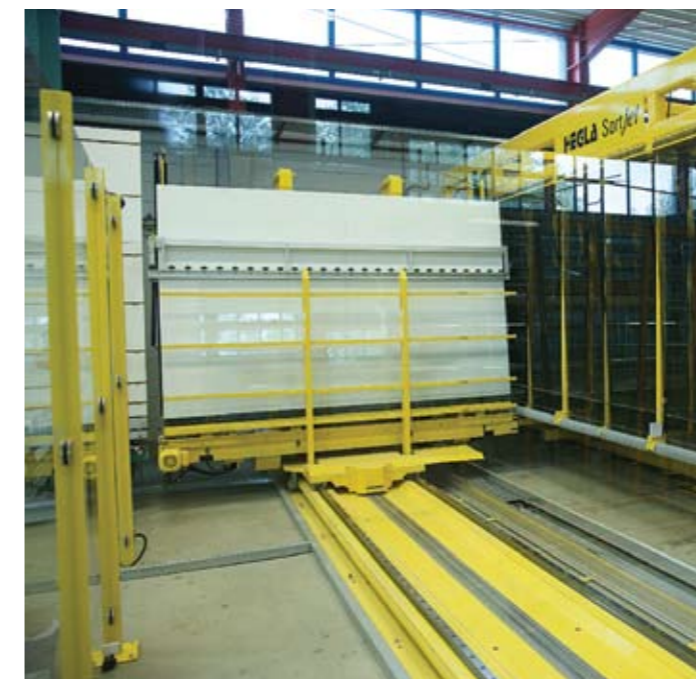
Fig. 01: Direct linking of cutting and IG line: The sorting buffer's unloading shuttle passing on a sheet.
