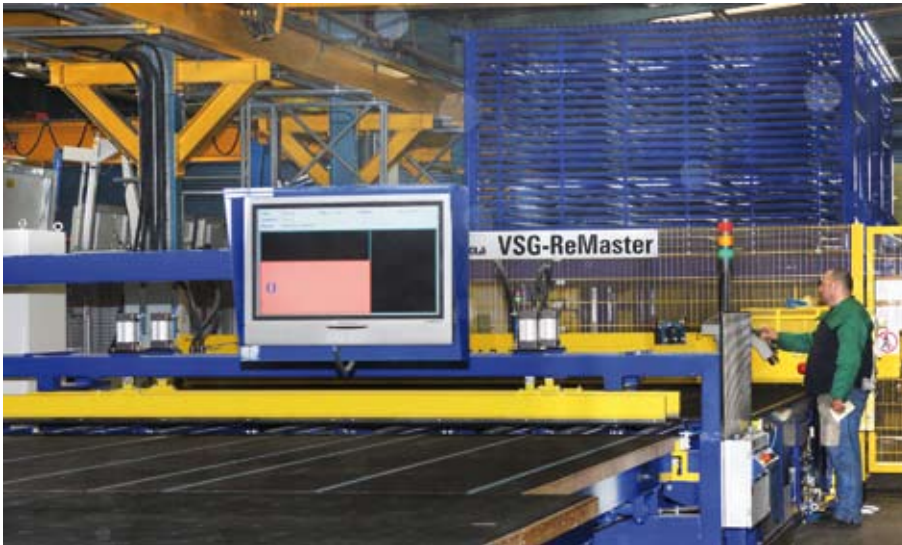
HEGLA cutting table for both laminated and float glass, with the perfectly integrated HEGLA Remaster sub-plate storer. Storer and cutting line are controlled by ALBAT+WIRSAM's XOPT-ON software.
