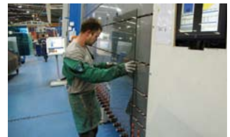
The brand new BYSTRONIC IG-Line, using LENHARDT's TPS warm-edge system, produces EVERSEAL™ insulating glass up to widths of 5 meters, especially for the commercial market. The giant line is controlled by ALBAT+WIRSAM ToolTV production management software.
