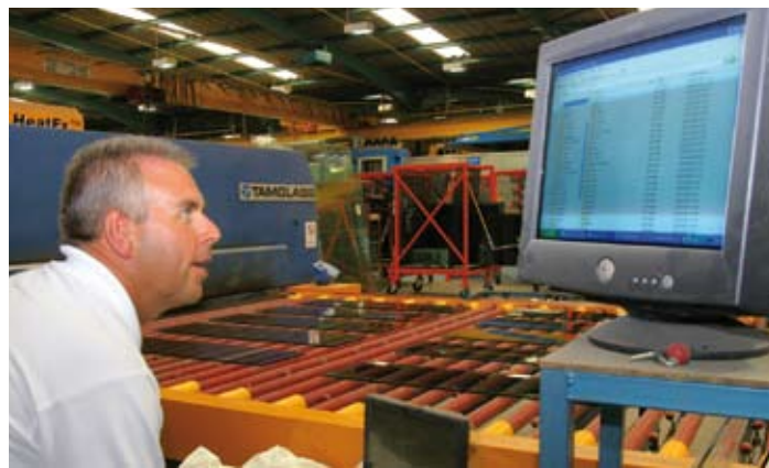
State-of-the-art and pretty fast: The high-performance TAMGLASS tempering furnace. The tempering process is supported by ALBAT+WIRSAM ToolTV-TG control stations - every sheet to be tempered is registered via barcoding and correctly forwarded to the next processing machine.
