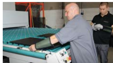
The new Giardina Paintline, which opaquely coats the spandrels in roller-coating technique.
