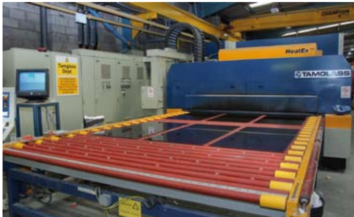
State-of-the-art and pretty fast: The high-performance TAMGLASS tempering furnace. The tempering process is supported by ALBAT+WIRSAM ToolTV-TG control stations - every sheet to be tempered is registered via barcoding and correctly forwarded to the next processing machine.
