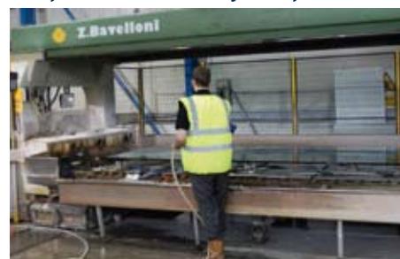
The BAVELLONI CNC processing centre for shapes and free-form shapes is fed online with processing data in new CAM-DXF format.
