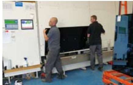
The brand new BYSTRONIC IG-Line, using LENHARDT's TPS warm-edge system, produces EVERSEAL™ insulating glass up to widths of 5 meters, especially for the commercial market. The giant line is controlled by ALBAT+WIRSAM ToolTV production management software.
