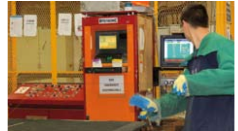
A+W control station XTV: This visualizing tool shows the employee at the breakout table breakout pattern and rack location, thus ensuring that glass is available at the tempering furnaces and the IG-line in the correct sequence.
