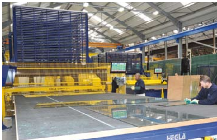
Both cutting lines are equipped with Hegla ReMaster storers that hold the valuable residual glass sheets which will be added to the optimisation real-time, controlled by A+W's XOPT-ON optimization software. The Float ReMaster (upper left) stores up to 35 residue plates, the Lami-ReMaster, visible in the background, 20 residual laminated glass sheets.
