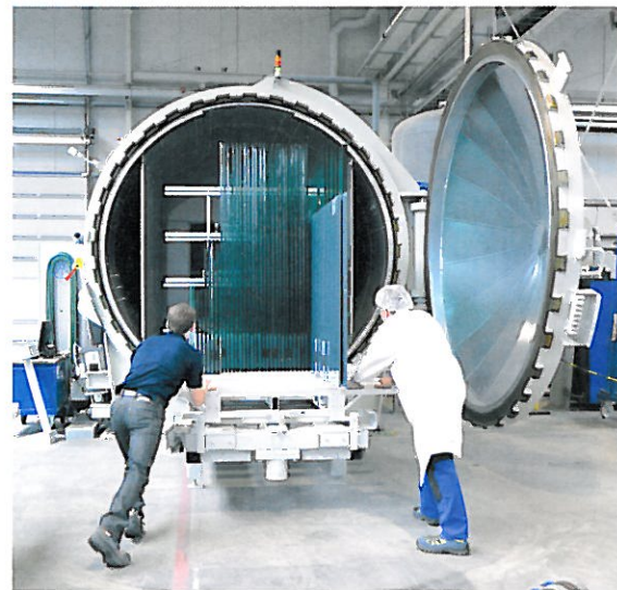
▲ Laminated glass production is comprehensively networked. The Autoclave is used for bigger tasks - like all machines at Sencoglas Glastechnik, it can handle sheets of up to 6 x 2.8m.
