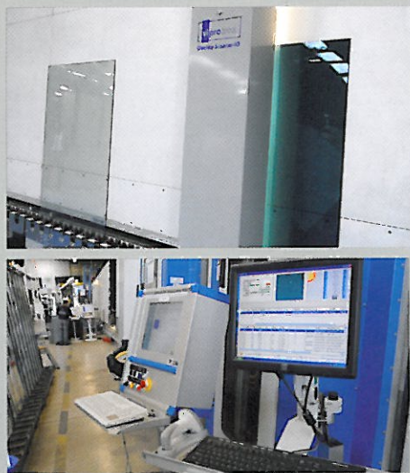
The VIPROTRON quality scanner reports breakage via the machine-related 'interlayer' A+W PANDRAMA to ALBAT+WIRSAM's production control system. The line 'knows' that the dirty or damaged sheet and its counterpane will be removed from the line and the following sheet pair is produced instead.
