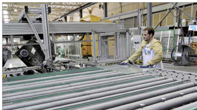
Left: XTV at the breakout table. The visualization tool is part of the A+W production software and displays cutting pattern and required production sequence – valuable assistance for the employee who breaks the lites before they go to the seamer.
