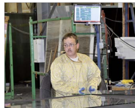
Left: XTV at the breakout table. The visualization tool is part of the A+W production software and displays cutting pattern and required production sequence – valuable assistance for the employee who breaks the lites before they go to the seamer.
