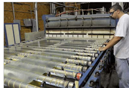
Automatically seamed and washed, a load of panes is fed to the Tamglass furnace
