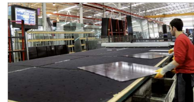
Always in view: XTV on large screen at the breakout table. The visualisation tool shows cutting pattern and rack allocation and thus helps to avoid expensive mistakes.
