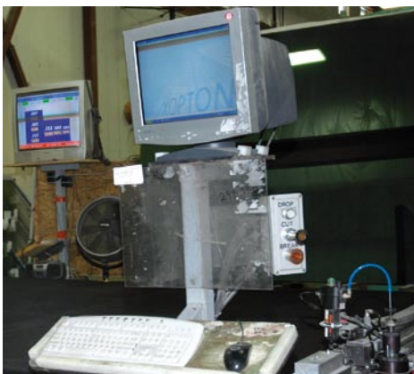
Remakes online in real time: XOPT-ON online control allows trouble-free cutting. Large scale CutTV breakout display visualizes breakout patterns and stacking instructions.
